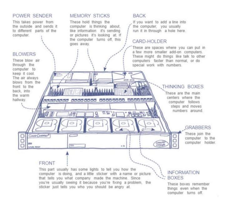
Word Bank: Fan, Hard Drive, CPU, RAM, Plug (Power Source)
